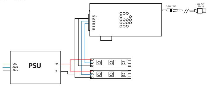
Each SPI Ground wire must be the same length as the Data wires per output, to prevent timing issues. Minor differences in length due to uneven stripping of the wires should not cause any problems.
