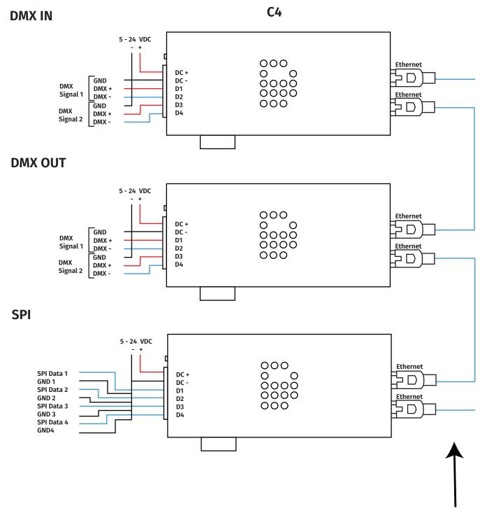
DiGidot C4 contains a small network switch so that the devices can be daisy chained for more output. Do not daisy chain more than 5 DiGidot C4 together.
